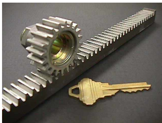
Figure 17: Steel gear and rack cut with an abrasive water jet
