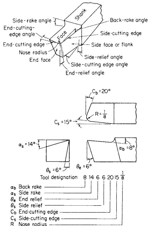
**Fig. 13.4.11** Standard nomenclature for single-point cutting tools.
