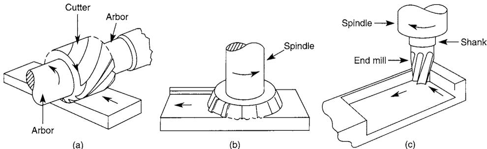
**Fig. 13.4.15** Basic types of milling cutters and operations. (a) Peripheral milling; (b) face milling; (c) end milling.
