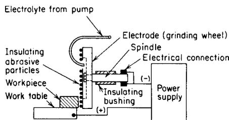
Fig. 13.4.23 Schematic diagram of the electrochemical grinding process.
