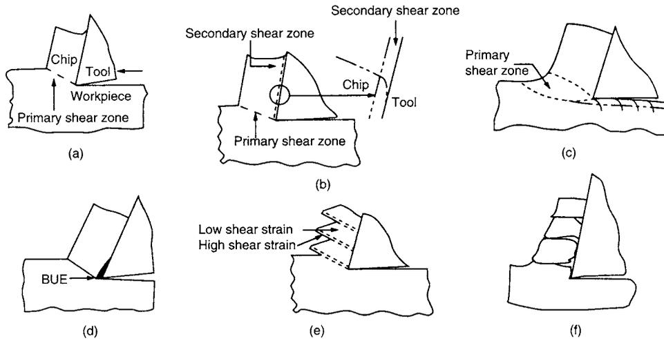
**Fig. 13.4.4** Basic types of chips produced in metal cutting: (a) continuous chip with narrow, straight primary shear zone; (b) secondary shear zone at the tool-chip interface; (c) continuous chip with large primary shear zone; (d) continuous chip with built-up edge; (e) segmented or nonhomogeneous chip; (f) discontinuous chip. (Source: After M. C. Shaw.)
