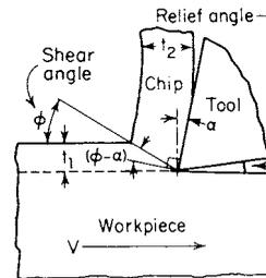
Fig. 13.4.2 Basic mechanics of metal cutting process.
