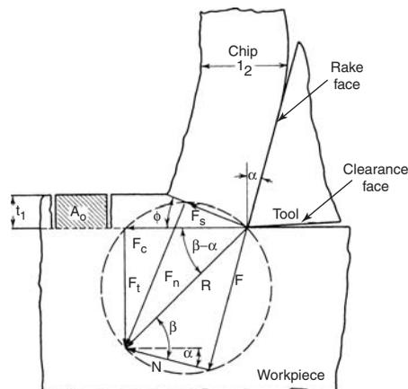
Fig. 13.4.3 Force system in metal cutting process.
