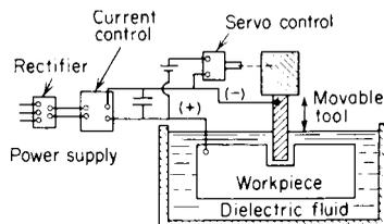
Fig. 13.4.20 Schematic diagram of the electric-discharge machining process.
