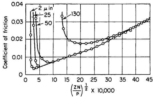
Fig. 13.5.2 Effect of surface texture on friction with hydrodynamic lubrication using a flat slider on a rotating disk.  $Z$  = oil viscosity, cP;  $N$  = rubbing speed, ft/min;  $P$  = load, lb/in<sup>2</sup>.
